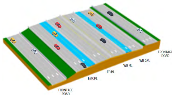
TYPICAL SECTION SEGMENT 1
