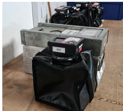
The heavy metal vault used beginning in 2005 is replaced in 2016 with a light-weight plastic bag with a locking mechanism.
