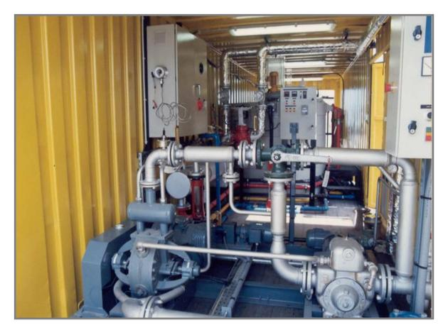
Mobile plant for manufacturing asphalt emulsions
